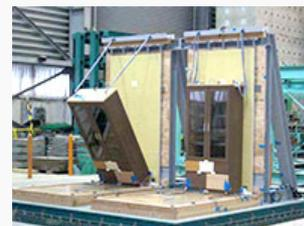
Testing in a vibration simulator
